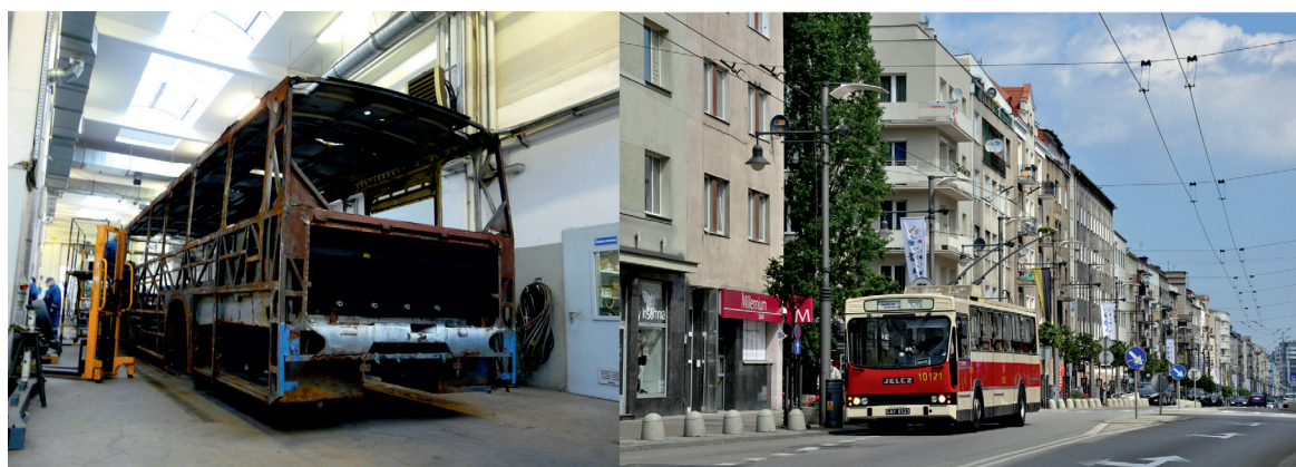
Figure 3. The condition of the Jelcz 120MTE trolleybus during the reconstruction in 2012 and after the reconstruction in 2018 (left photo by Marcin Połom, right photo by Karol Grzonka)
